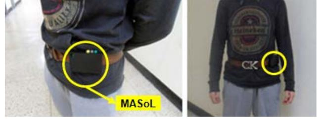
Fig. 4. MASoL has been worn by the patient. For avoiding installation error, we fixed the direction and location of the device to waist. User controls the device by three buttons(turn on/off, reset, resume etc.) above it.
